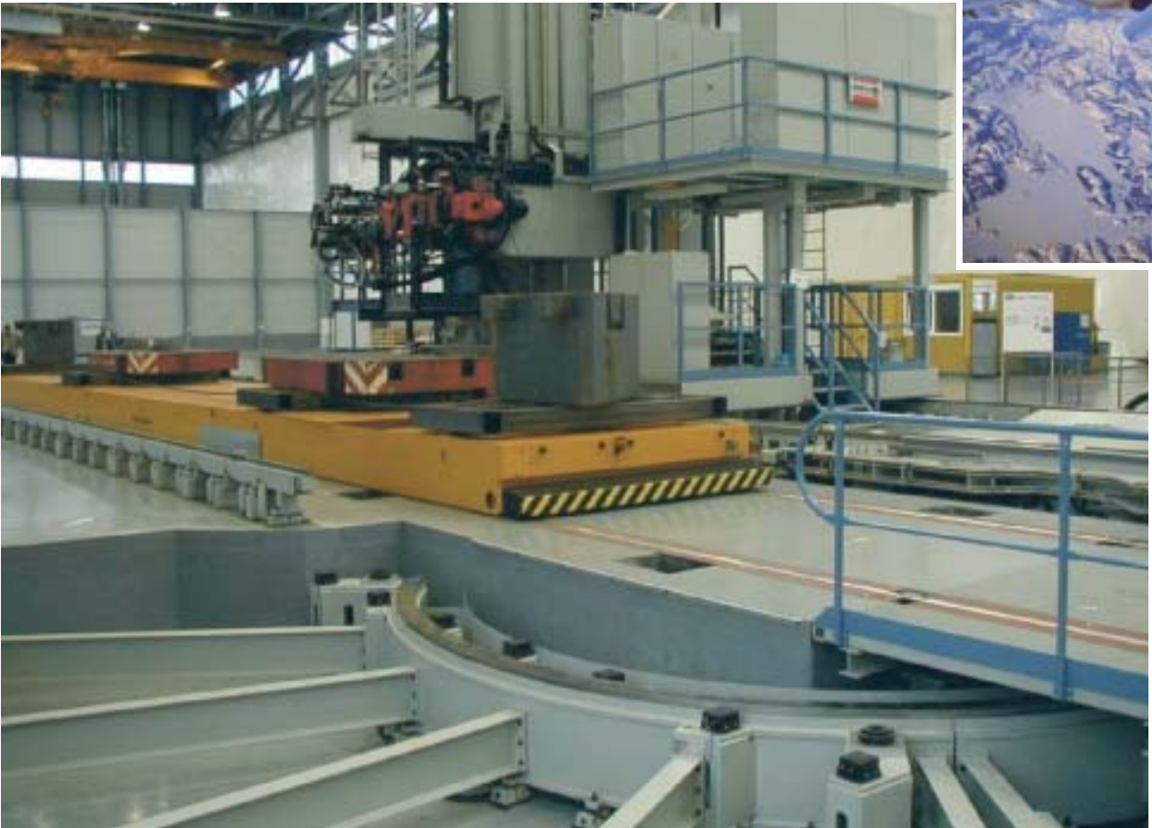
Carriage (21 m) for transportation of aircraft tail units into a riveting machine.
