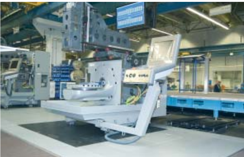
Deckel MAHO at Seebach (Germany). Flow production on high precision assembly platforms. During indexing between the stations the skid platforms will be lifted by air cushions, transferred and afterwards rested and levelled at 4 centring units. A big challenge was to constantly provide the machines with compressed air and electricity; both during the transportation process and at their assembly position.
