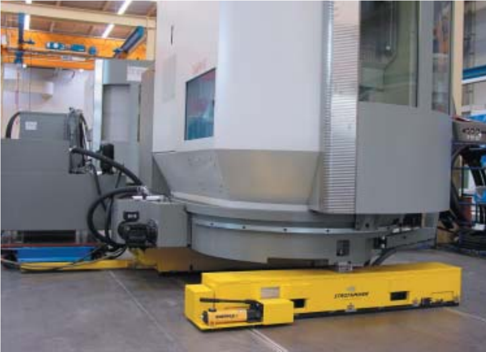
20 tons Milling Machine in pulse production. Drive cart powered and data connected via inductive power supply. Tailored follower cart with hydraulic power pump.
