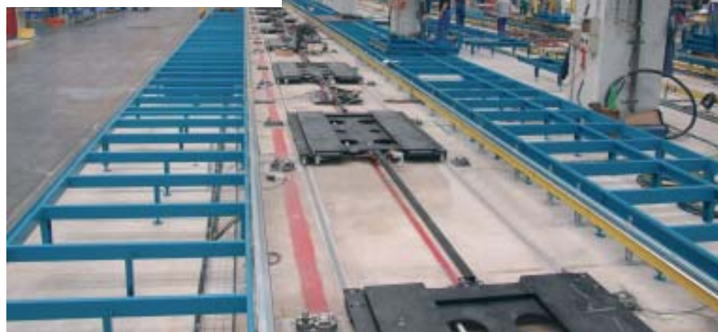
Deckel MAHO at Seebach (Germany). Flow production on high precision assembly platforms. During indexing between the stations the skid platforms will be lifted by air cushions, transferred and afterwards rested and levelled at 4 centring units. A big challenge was to constantly provide the machines with compressed air and electricity; both during the transportation process and at their assembly position.
